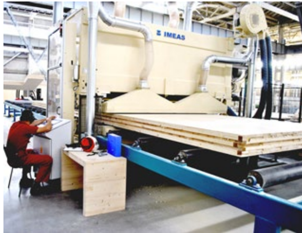
Latvian company „Cross Timber Systems” Ltd was the first in Northern Europe that started producing cross laminated timber construction panels or CLT
