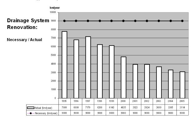
Figure 3.3-1: Renovation of drainage systems - Actual status and necessity within 10 years period (1995 - 2005).
